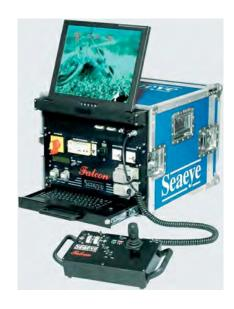
The Seaeye Falcon is a compact remotely operated vehicle suitable for a variety of observation and inspection tasks. It is idealy suited to rig support eyeball operations where it sets the highest standards including
