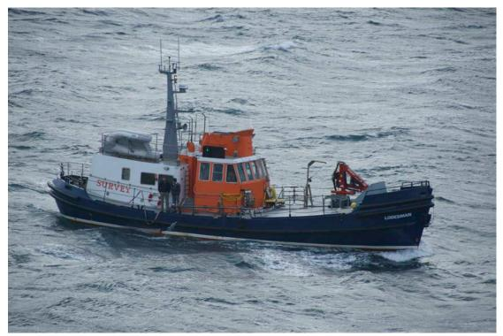
Overall design was by Burness Corlett & Partners to Lloyds specifications. The hull is steel and superstructure G.R.P.
